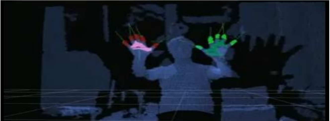
Figure 11: Capturing fingers using the Kinect's 3D sensors
