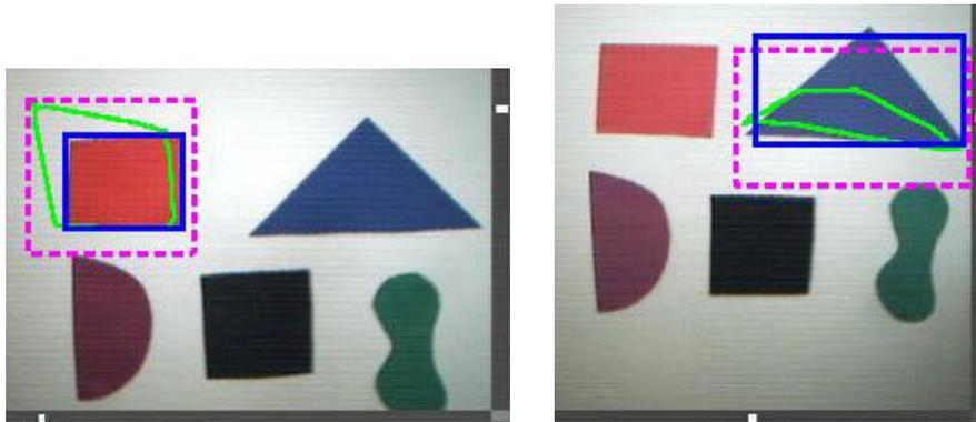
**Figure 8.** Sample fusion results for Experiment 1. Eyetraces are shown in green, the gaze-only solution is shown as a dashed magenta box, and the output of the fusion algorithm is in blue. Using the color structure of the images the fusion algorithm was able to overcome these inaccurate eyetraces to achieve an excellent solution.
