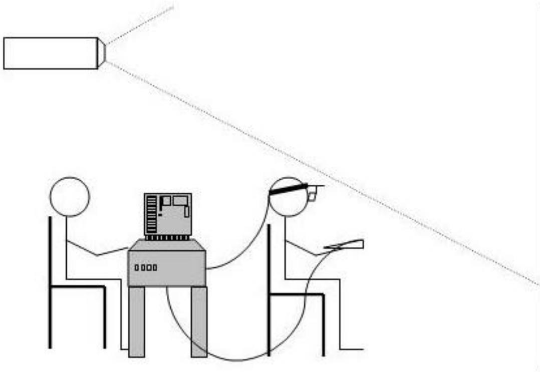
**Figure 1.** Experimental setup. An experimenter (left) controlled an overhead LCD projector displaying stimuli on a wall in front of the subject.
