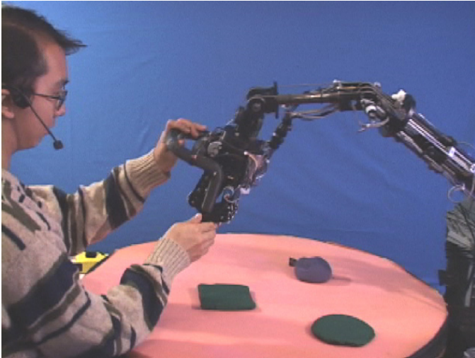
Fig. 2. Ripley’s motions can be trained through direct manipulation. The motor controllers are placed in a “anti-gravity” mode so that a human trainer can effortlessly guide Ripley through natural motions. Motion trajectories recorded during training are processed by interpolation algorithms that are combined with visual guidance to generate novel motion trajectories.
