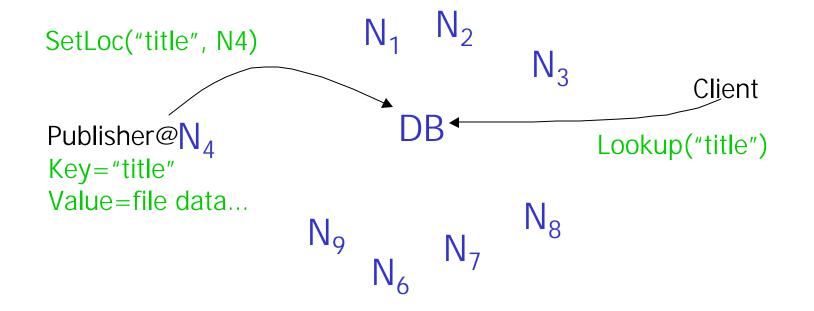
Simple, but O(N) state and a single point of failure
