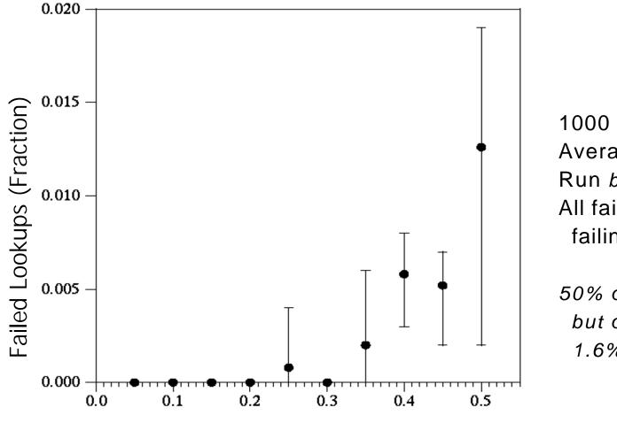
1000 DHT servers Average of 5 runs Run *before* stabilization All failures due to replica failing
