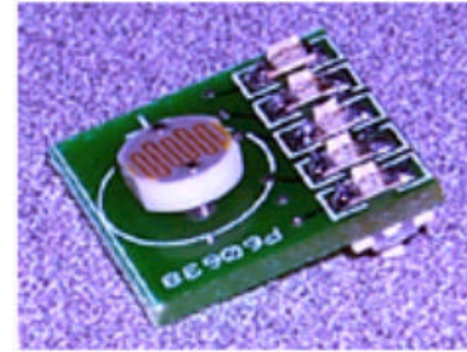
Light sensor & LED top layer
