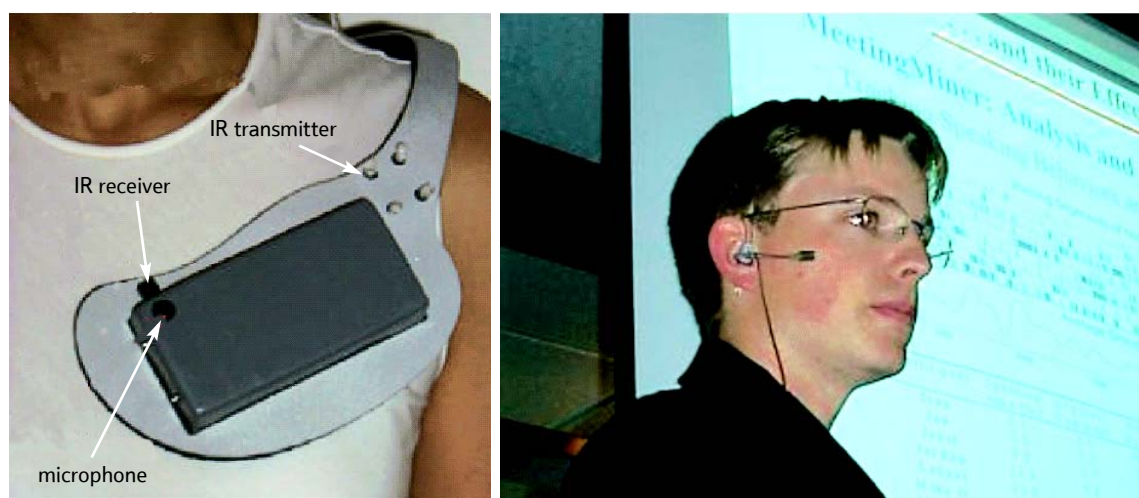
Fig 1 Measuring social interactions — left, the shoulder mounted sociometer; right, the headset connected to a PDA or mobile telephone.
