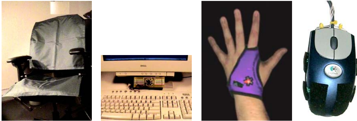
Fig 1 Various sensors can capture postural, facial, skin-surface, and gestural changes that carry affective information. From left to right: chair with Tekscan pressure sensors, BlueEyes camera, Galvactivator skin conductivity sensor, and pressure mouse.
