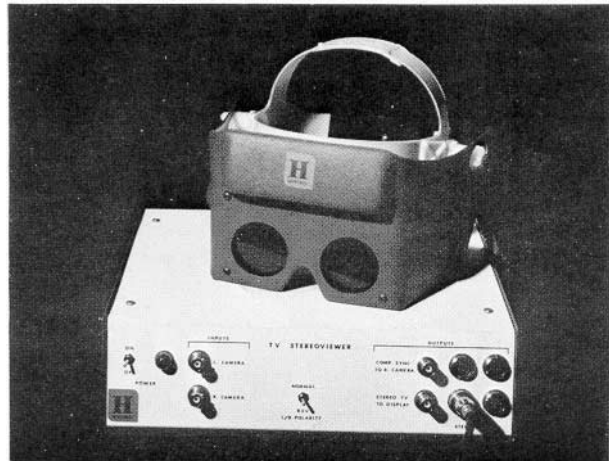
Figure 3. The PLZT glasses and electronic controller box.
