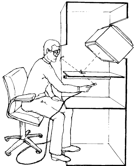
Figure 1. A cutaway view of the work station, showing the view through the half silvered mirror of the video monitor and user's hand.
