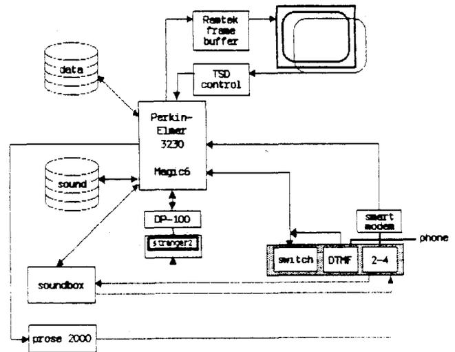
Figure 2: Hardware configuration used in Phone Slave.
