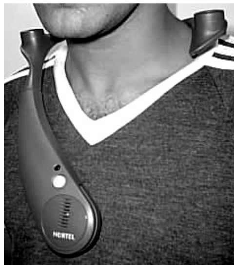
Figure 2: The wearable audio device, the Soundbeam Neckset , with directional speakers and microphone
