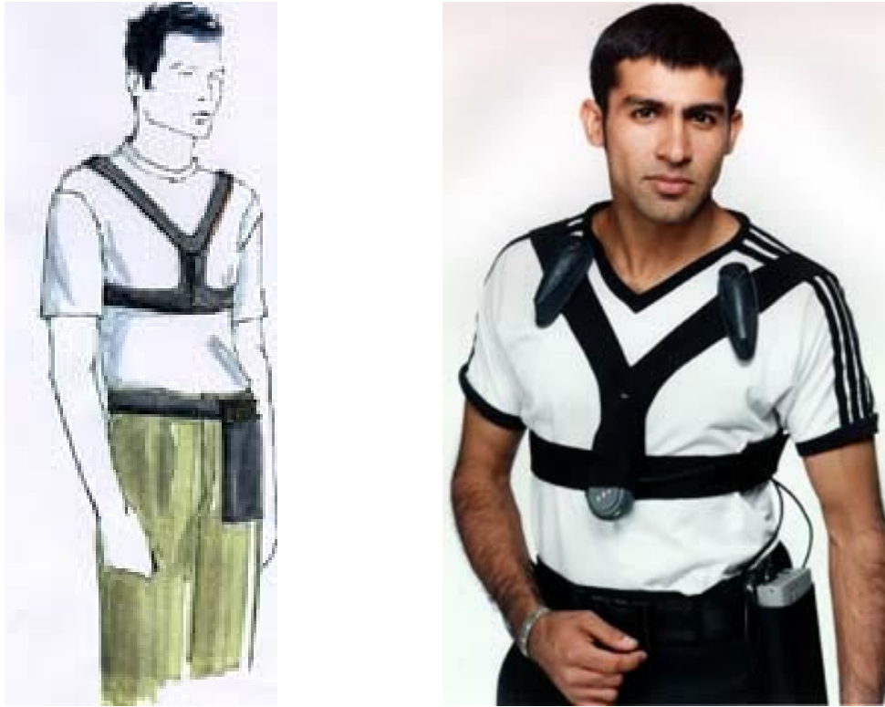
Figure 3.4: The Radio Vest , conceptual design and final implementation of an outdoor wearable configuration with clip-on directional speakers and powered microphone.
