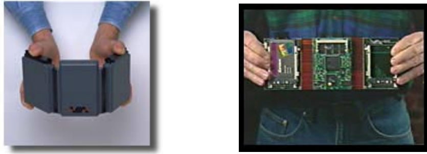
Figure 6.5: The VIA Wearable from Flexipc, shown here with the flexible circuit-board.
