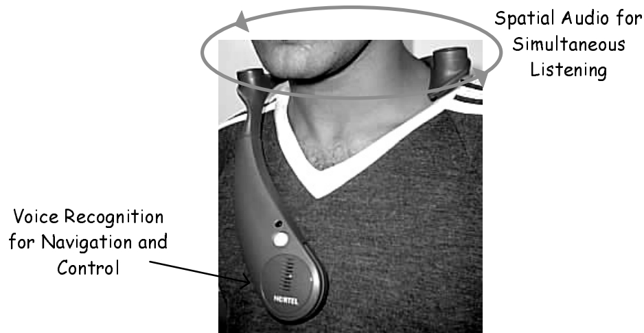
Figure 3.3: The Nortel SoundBeam Neckset , the primary wearable audio device adopted in Nomadic Radio for inter-office use. The directional speakers are utilized for rendering spatialized audio to the listener, and a directional microphone allows speech recognition.
