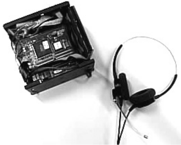
Figure 6.4: The Lizzy wearable platform developed at the MIT Media Lab, shown here configured with audio I/O for Nomadic Radio .
