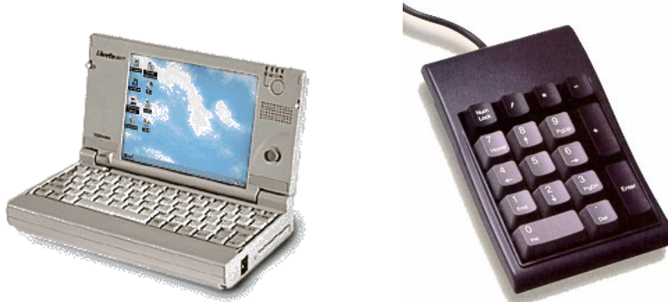
Figure 4.5: A numeric keypad connected to a networked Toshiba Libretto 50CT mini-notebook PC. This is useful for providing tactile feedback when speech is not feasible.
