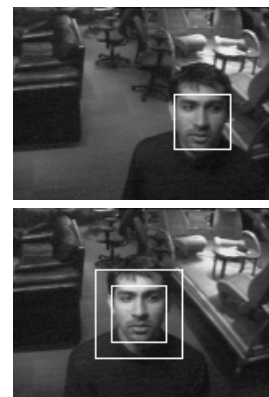
Figure 4: Detecting a person glancing at an article and stepping closer to see more. By gazing at the camera for a longer duration, a person allows the system to capture his face.
