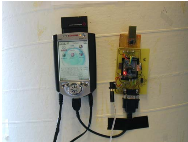
Figure 4-3 Sound Collecting Module (SCM): From left to right: PDA connected to TB
