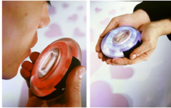
Figure 2-3: IDEO's kiss communicator device.
