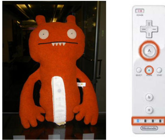
Figure 3-7: (1) The toy (Abima) with a Wii controller belly. (2) The Wii remote controller with active buttons and LED's marked in red.
