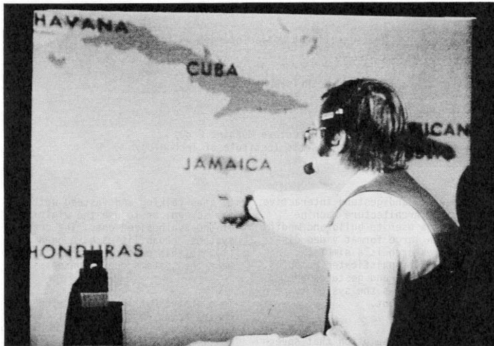
Figure 1: In running "Put That There", the user points at the large screen using a position sensing device strapped to his wrist. He speaks to the system through the head-mounted microphone.
