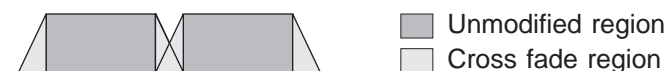
Figure 2: A linear cross fade between segments of the sampling method to reduce distortions.
