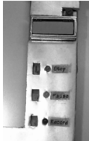
Figure 3-10: Version 1 Audio Notebook audio controls (record, pause, stop) are activated by dipping the pen inside them.
