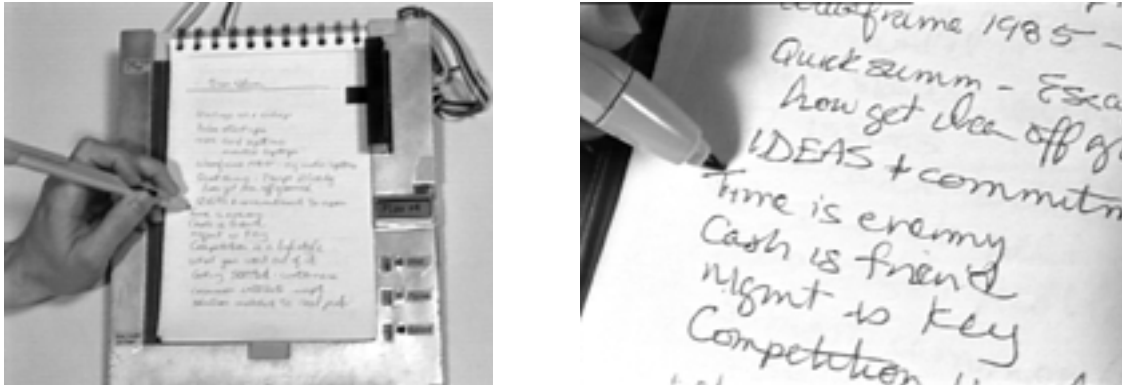
Figure 3-11: The user can randomly access different parts of the audio recording by pointing to a location in his/her notes (version 1 prototype).
