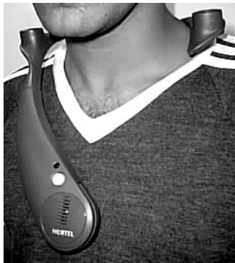
Figure 2: The primary wearable audio device for inter-office use, the Soundbeam Neckset , with directional speakers and microphone.
