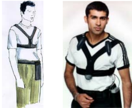
Figure 3: The Radio Vest , conceptual design and final implementation of an outdoor wearable configuration with clip-on directional speakers and powered microphone.
