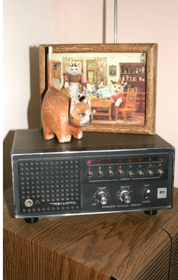
Figure 3-1: A 1970's era radio scanner uses simple toggle switch for channel inclusion in scan.
